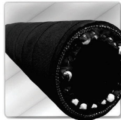
1 1/2" ID discharge hose. The ceramic balls are embedded in a black 60 duro high abrasion synthetic rubber.
