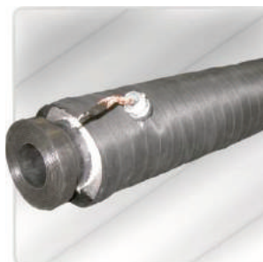
EPDM hose with heating wire, sponge insulation, c/w molded beaded ends.
