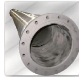
16" ID x 25 ft Oilfield Hose, c/w nipples & flanges 150# fix x floating.
