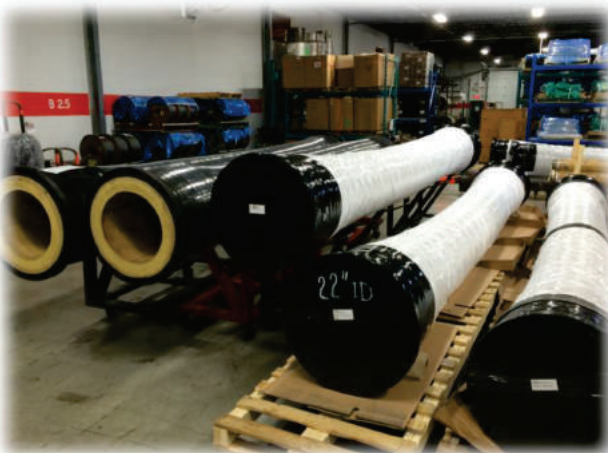
22" slurry hoses, pure gum tube, c/w built-in rubber lined nipples & flanges 150#.
